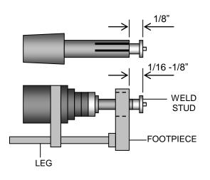
The weld chuck should be adjusted as shown. For longer studs, as much of the stud should be held as possible. This may require complete removal of the adjusting screw.
