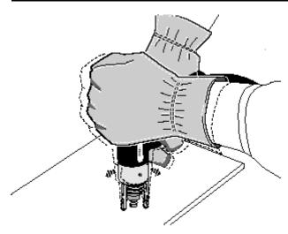
Place the weld gun perpendicular to the workpiece as shown. Apply pressure to the gun so the footpiece lies firmly on the workpiece.
