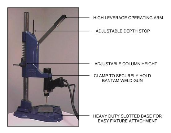
The heavy duty Cutlass drill stand is designed specifically for the Bantam stud welding gun. It will accept either of the CD welding guns, C8 or C10, or the A-58 ARC welding gun.
